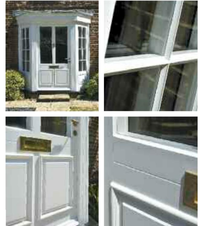
Kingston design front door finished in 'White' with 4mm single putty glazing and bolection moulding. Ironmongery from Samuel Heath includes an Extended Profile handle, Ring knocker and Medium sized letter plate in Polished Brass Unlacquered. The side window panels are also single putty glazed and feature 22mm true bars.
